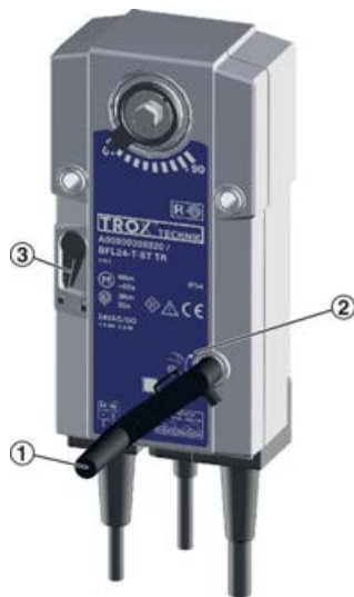
Fig. 205: Functional test (without power supply)
