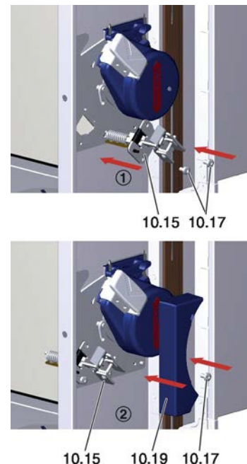
Fig. 161: Install the fusible link holder
